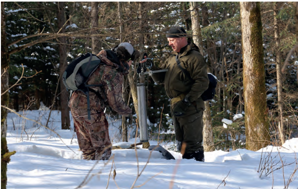
Figure 15. Snow surveys include taking samples with the snow-measuring cylinder, estimating its mass (depending on density and volume) and thickness.
