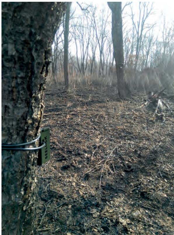
Figure 30. An example of setting trailcams on a tree.
