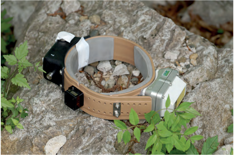
Figure 21. The collar Iridium Track M Collar 1D from Lotek, Canada with a fastened battery, a GPS block, Iridium and VHF transmitters and a drop-off.
